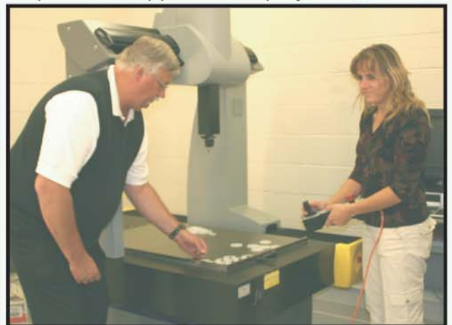
QA Director Rob Zancig (left) and QA Manager Aneta Cop diligently set up the CMM Machine.
